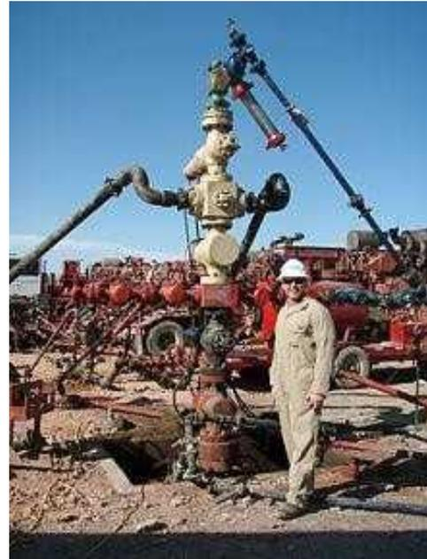
Figure 9 – Well Head, Fluids Being Injected
